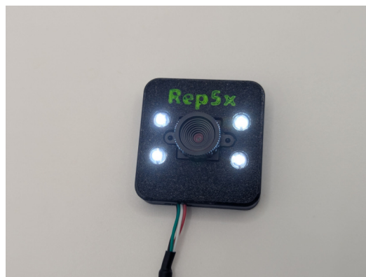
FIG. 5.12 The Rep5x Camera, a roughly €10.50 USB camera calibrator. Left: four white LEDs soldered directly to the OV9726 board for even nozzle lighting. Right: the finished, magnet-mounted module, read live by the browser calibrator.
